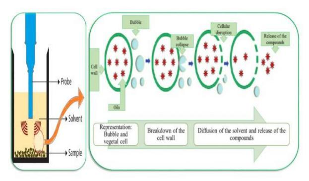
Figure 3. The principle of acoustic cavitation. Modified from Soria and Villamiel
