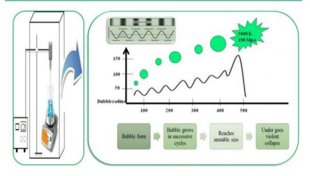
Figure 4. Graphical representation of cavitation-bubble collapsing and releasing plant material in three steps.
