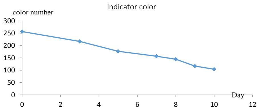
**Figure 6.** Color Number of Indicator in Chicken Meat Samples during 10 Days of Storage at Refrigerated Temperature (4°C)
