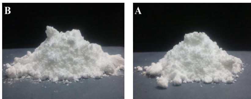
**Figure 2.** Spray dried powder of vitamin D<sub>3</sub> and calcium stearate (A) and vitamin D<sub>3</sub> and calcium carbonate (B) microcapsules.
