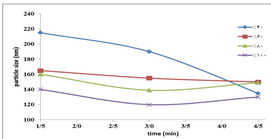
**Figure 1.** The effect of sonication time and intensity on emulsion droplet size.
