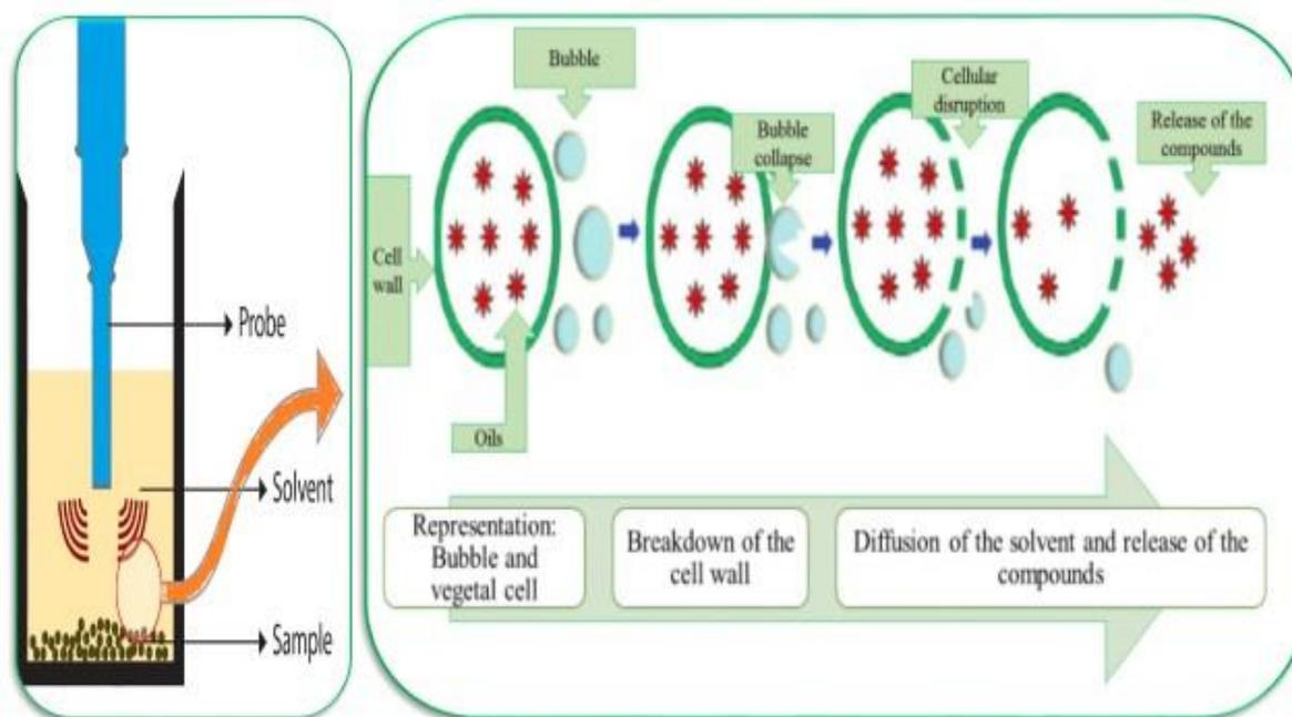
Figure 3. The principle of acoustic cavitation. Modified from Soria and Villamiel
