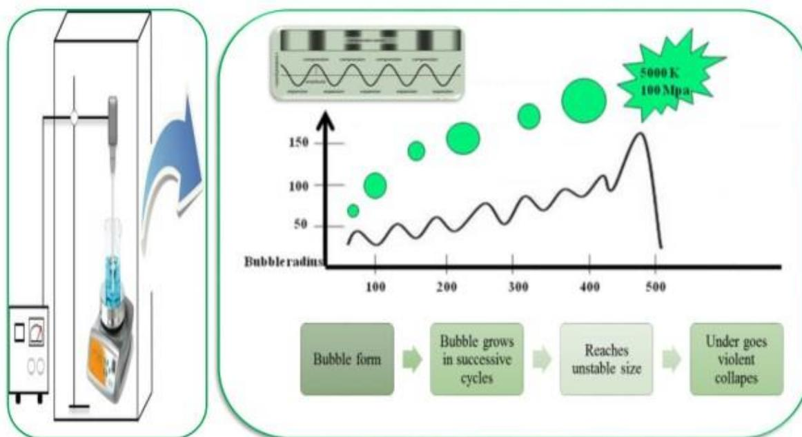
**Figure 4.** Graphical representation of cavitation-bubble collapsing and releasing plant material in three steps.
