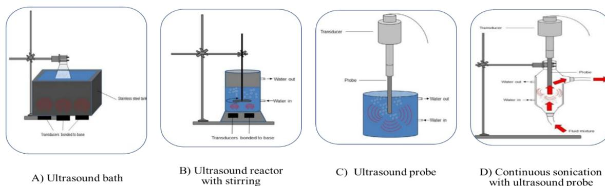
**Figure 2.** Commonly used ultrasonic systems
