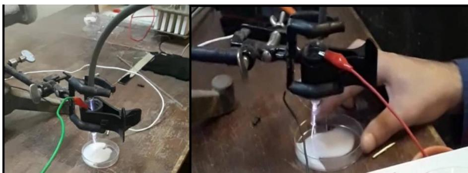
**Figure 2.** Exposition of contaminated milk samples with cold plasma
