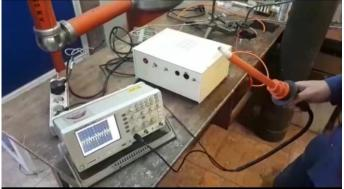
Figure 1. A view of the atmospheric cold plasma generator.
